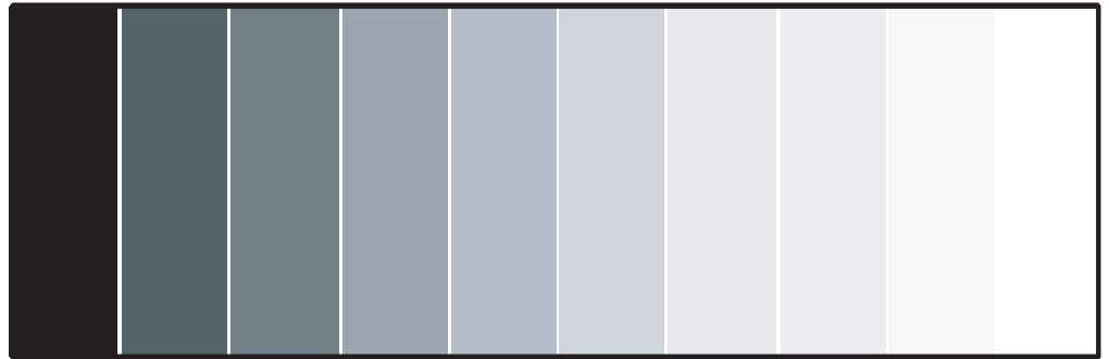
Figure 4-3. Typical Gray Bar Pattern for Adjusting Contrast
